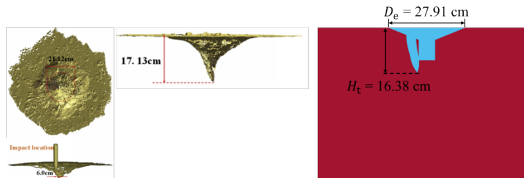
(b) Results comparison for Case 1 (low speed): Left: experimental result; Right: theoretical prediction
