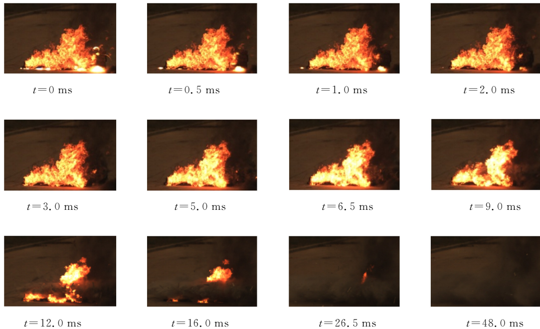
图 14 冷激波灭火实验过程 Fig. 14 Fire extinguishing process by cold shock extinguishing bomb
