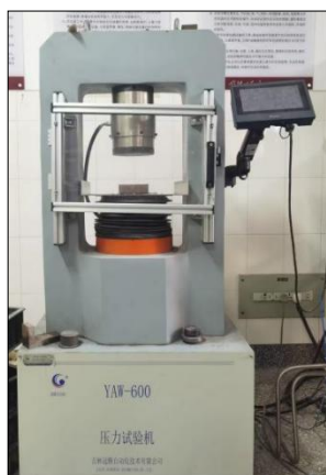
(a) Static pressure testing
