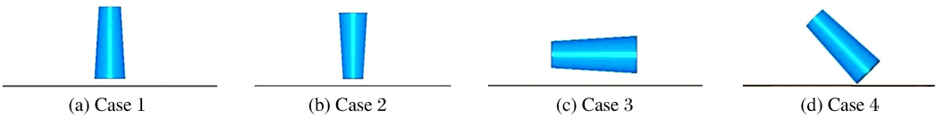
图 2 带舱大型战斗部跌落试验工况 Fig. 2 Fall test conditions of large warhead in cabin
