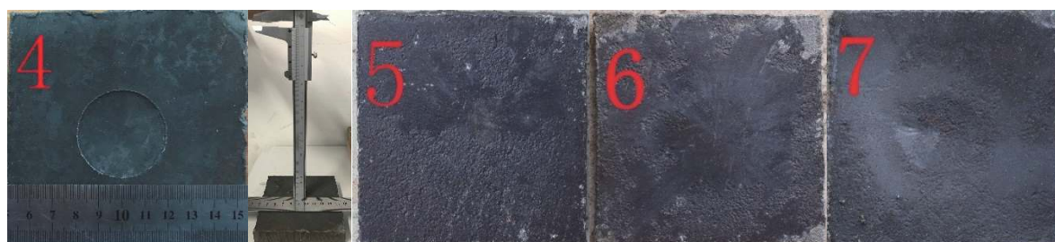
图 6 非接触爆炸试验后被发装药的见证板变形 Fig. 6 Deformation of the witness plates under the acceptor with non-contact explosion
