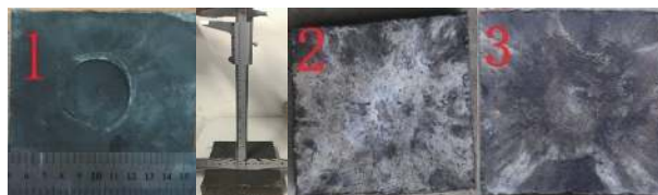
图 5 接触爆炸试验后被发装药的见证板变形 Fig. 5 Deformation of the witness plates under the acceptor with contact explosion
