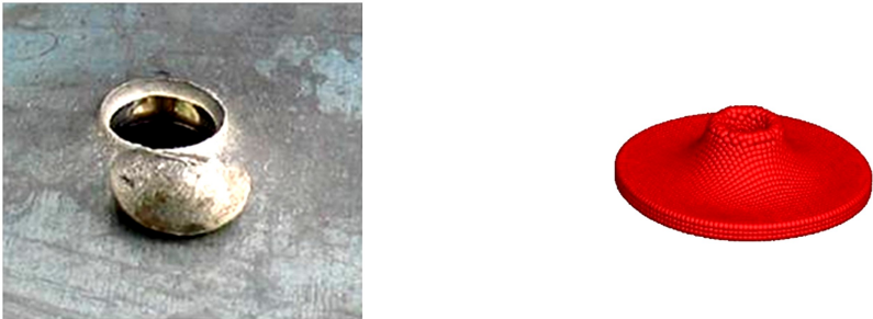
图 6 半球形弹头撞击 6 mm 单层靶板实验和数值模拟对比 Fig. 6 Experiment and numerical simulation of 6 mm plates impacted by hemispherical-nosed projectile
